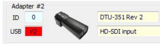
In USB-2 mode, the DTU-351 is visible in DtInfo and VPD data can be read, but the DTU-351 cannot transfer HD-SDI or other data at all.
