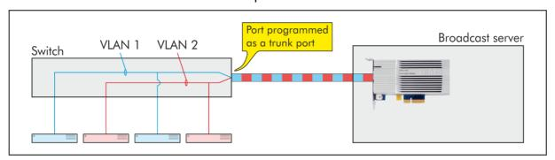
DekTec network adapters support this way of working. Multiple VLANs can be configured, and in Windows each of them will show up as a separate connection in Control Panel's Network Connect window. From the DekTec SDK it is straightforward to transmit or receive TS-over-IP streams to o a specific VLAN.
