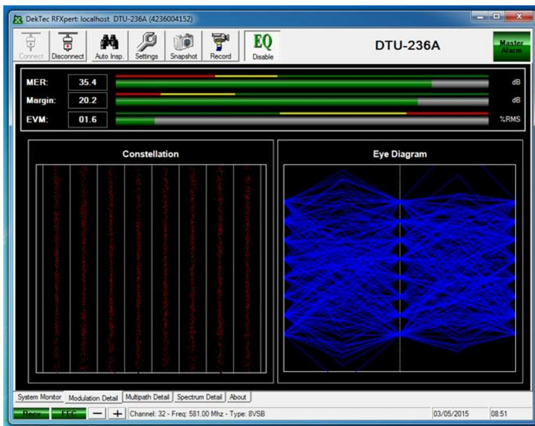
Figure 43. MER and Modulation Detail with EQ ON
