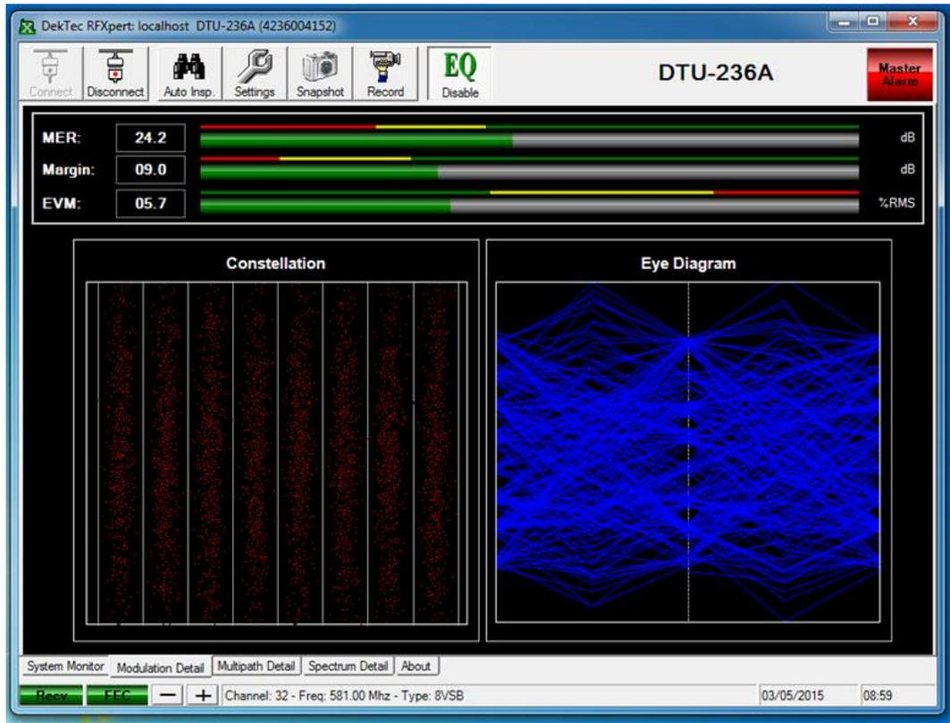
Figure 44. MER and Modulation Detail with EQ DISABLED
