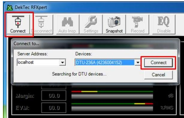
Figure 5. Connecting to an RF Probe
