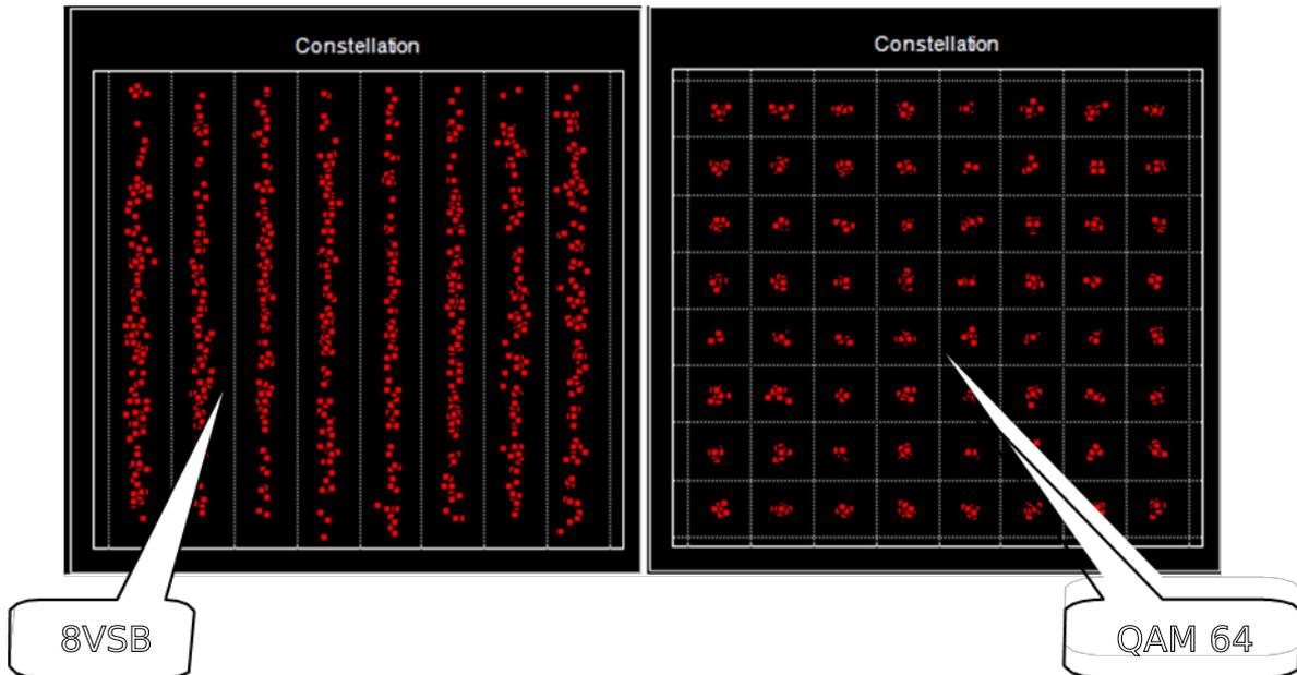
Figure 25. 8VSB and QAM Constellation Displays
