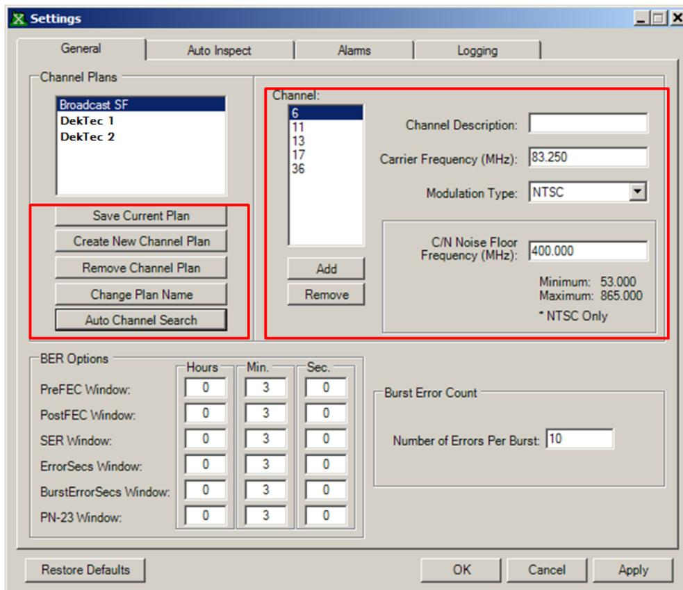
Figure 14. Modifying and Saving Channel Plans
