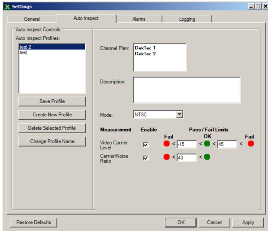
Figure 49. NTSC Parameters within Auto Inspect
