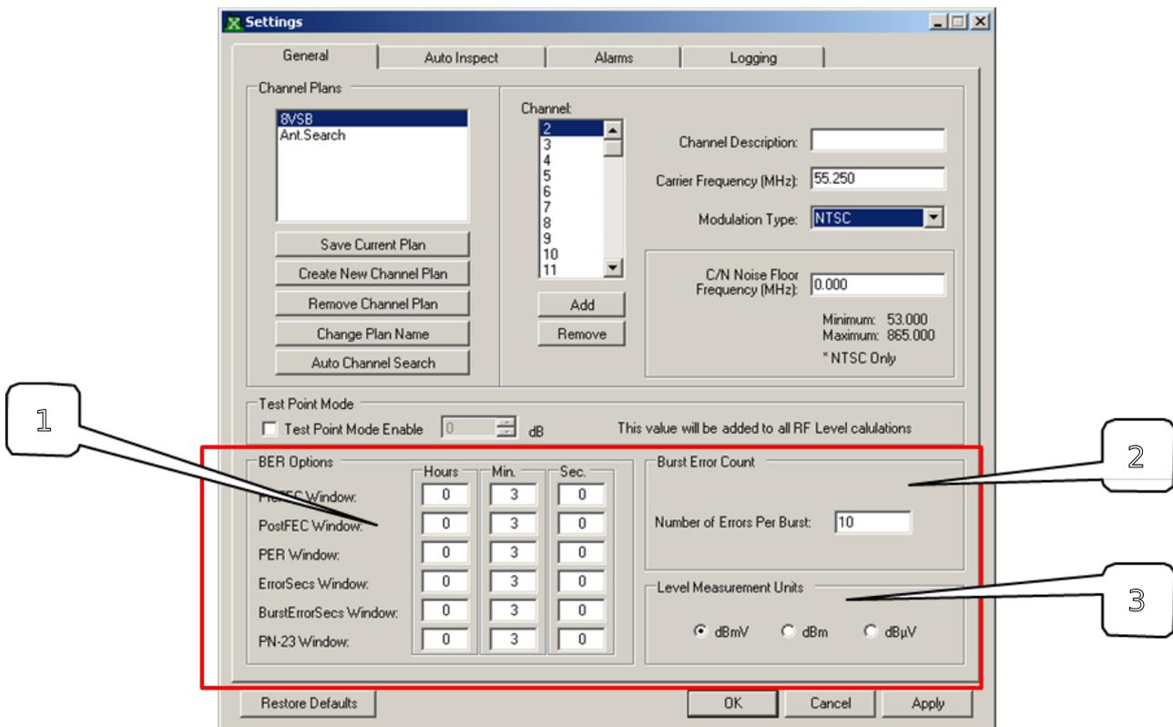
Figure 16. Additional Measurement Settings
